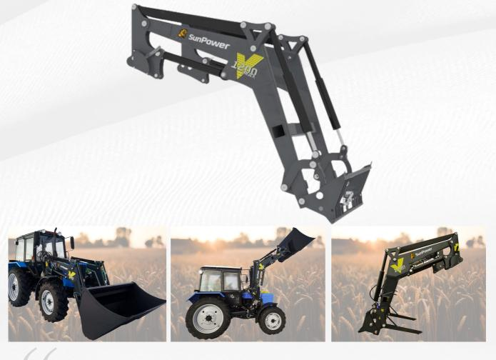
The «Sunpower» max 1200 front loader is a multi-purpose tool with improved characteristics for attachment to class 1.4 tractors of domestic and foreign production. It perfectly handles the tasks of loading and unloading various fine materials, such as crushed stone, sand, gravel, as well as single-piece and bulky loads.
