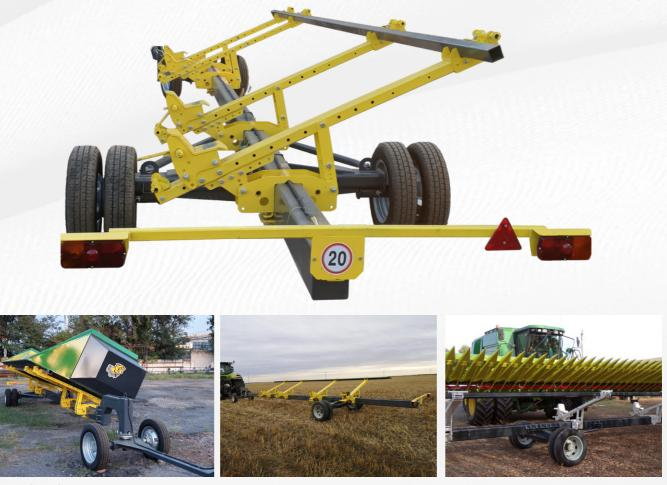
The «Carrello 2 Axes» dual-axle trailer is designed for transportation of any type of grain headers weighing up to 5 tons and with a cutting width of up to 12 m on dirt roads and public roads aggregated with a combine.
