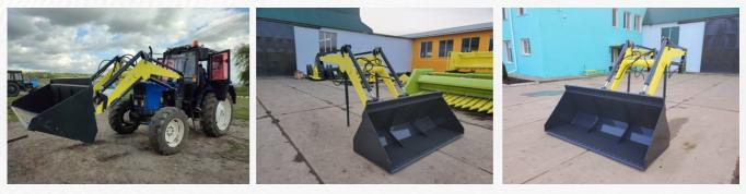
The «Strong» front loader is a multi-purpose tool for attachment to class 1.4 tractors of domestic and foreign production. It perfectly handles the tasks of loading and unloading various fine materials, such as crushed stone, sand, gravel, as well as bulky and single-piece loads.
