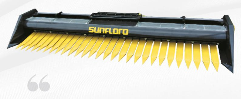
The «Sunfloro Shaft» header is a prefabricated structure based on a platform frame to which the pulling shaft, cutting device, reel, auger, fender plates and a planetary cutting device drive are fixed. The header is driven by a propeller shaft from the combine PTO to the drive shafts, from which rotation is transmitted through chain drives and overload clutches to the auger shaft on the left and the reel shaft on the right.
