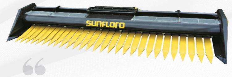
As the header moves across the field, the pointed ends of the crop lifters accurately separate the crop into rows regardless of the combine direction. The original prismatic shape allows them to easily penetrate the crop and separate it while maintaining the vertical position of the stalks.
